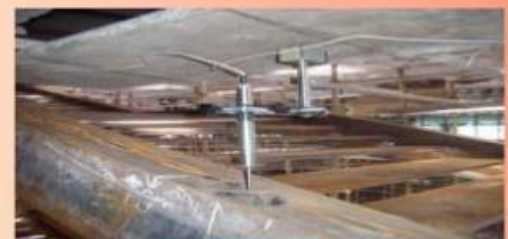
MEASUREMENT OF DEFLECTION BY LVDT
