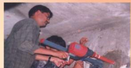
EXTRACTION OF SMALLER CORE SAMPLE FROM MEMBER
