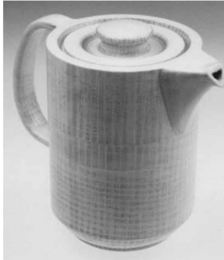
LOM model of a tea pot (Courtesy of Champion Machine Tools, Singapore)
