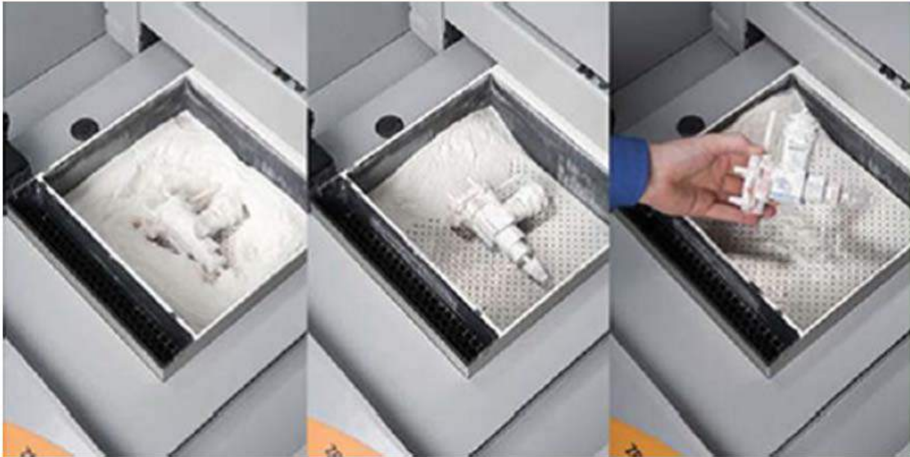
Automated powder removal using vibratory and vacuum assist in a ZCorp 450 machine (Courtesy Z Corporation)
