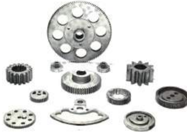
Fig. 1.4. Components manufactured by sintering
