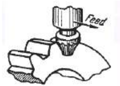
Fig. 1.16 Form milling by end mill cutter
