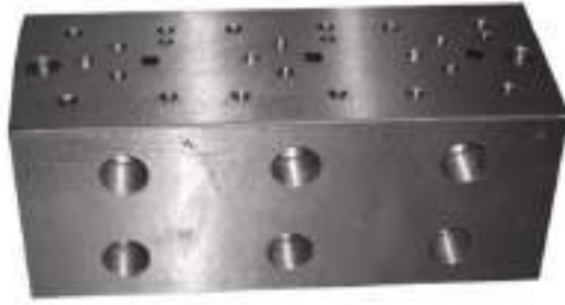
Figure 1.34 Manifold for three valves
