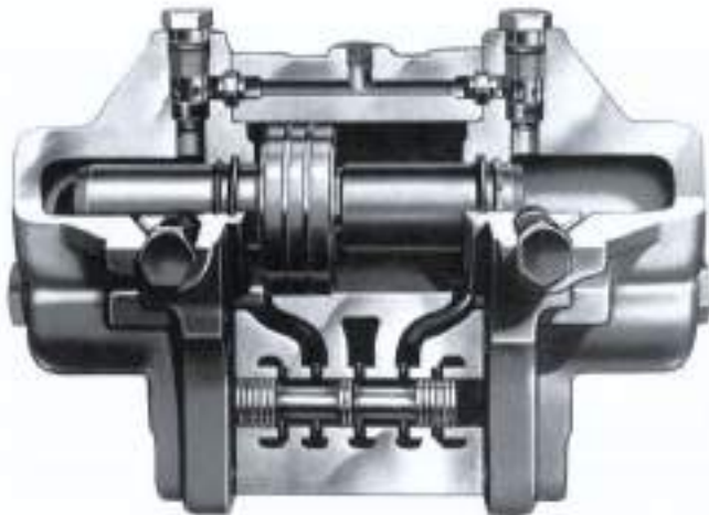
Oil flow paths of pressure intensifier.
