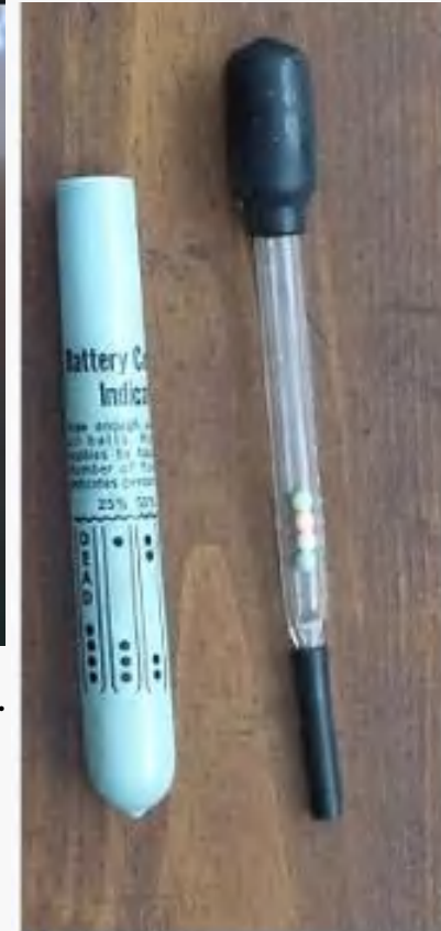
Battery condition indicator to measure the charge of the battery (~1985).
