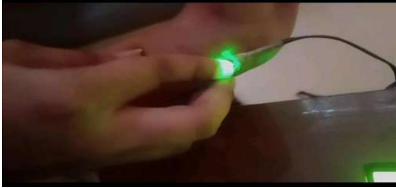
Measuring Pulse rate using the pulse sensor
